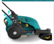
The lateral wheel of the sweeper in addition to activating the main brush, also activates a drive shaft connected to a fan. The ratio between the wheel and drive shaft creates strong suction, which picks up dust and channels it towards the filter.
